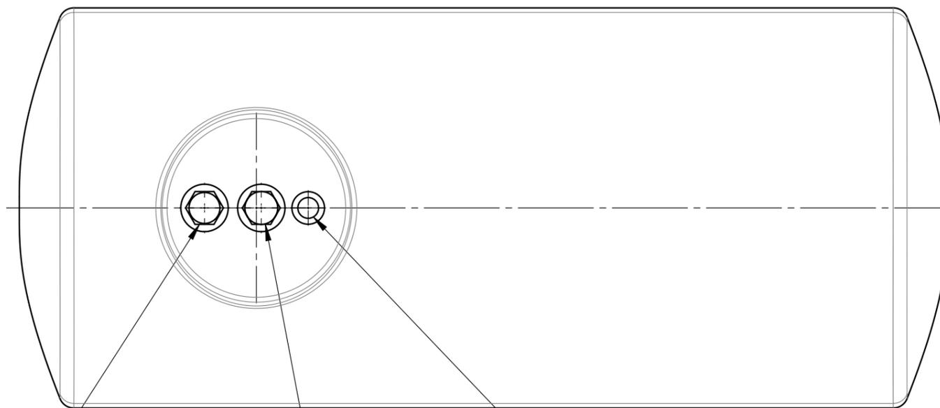
50mm female outlet    50mm Filling point    20mm Vent
